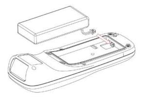
Figure 2-2 Diagram of replacing the Lithium-ion battery
