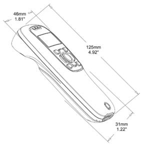
Figure 1-1 Dimensions of the terminal
