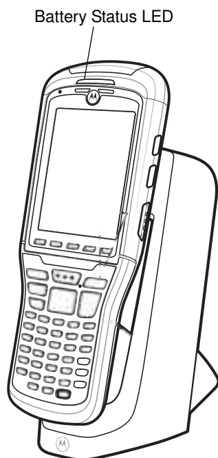
Figure 8-2 MC9500-K Battery Charging
