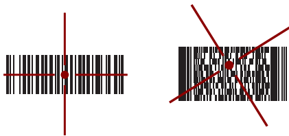
Figure 2-29 Imager Aiming Pattern: Bar Code Centered
