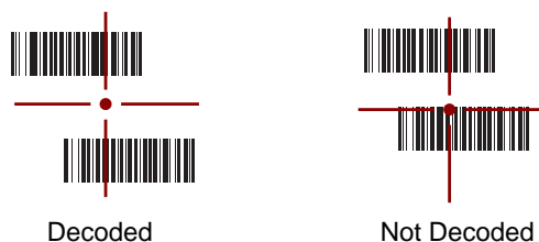
Figure 2-31 Pick List Mode with Multiple Bar Codes in Aiming Pattern
