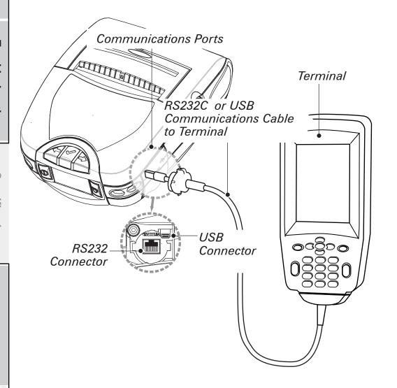
Figure 15- Connecting to a PC
