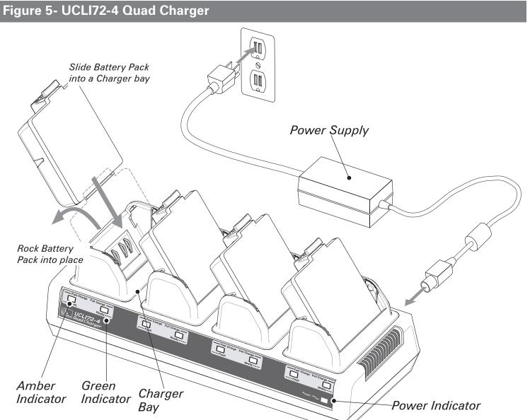
The UCLI72-4 Quad Charger is designed to charge up to four battery packs simultaneously. Charging times are as follows:
