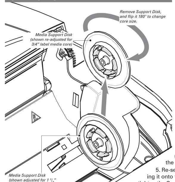
Figure 8- Adjusting the Media Core Diameter
