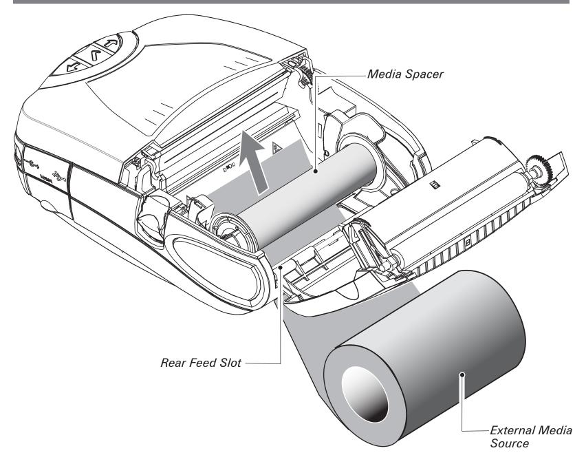
Refer to Figure 7.3. A P4T Series printer configured with the External Media option has a loading slot in the rear of the media compartment allowing you to use 4.0 in. (101.6 mm) wide fanfold or roll media from an external supply. The external supply must be designed such that it does not exert excessive drag as media is fed through the printer, which could result in distorted printing.
