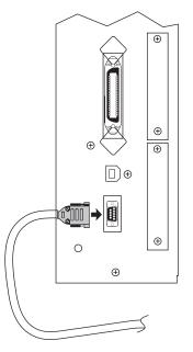
Figure 31 • Serial Connector
