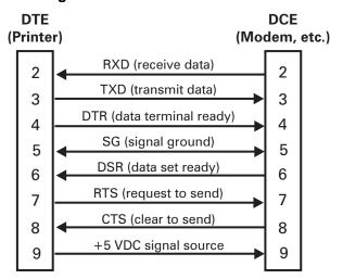
Figure 34 • RS-232 Connections
