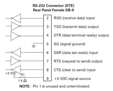
Figure 32 • RS-232 Connections
