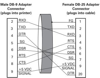
Figure 33 • DB-9 to DB-25 Connections
