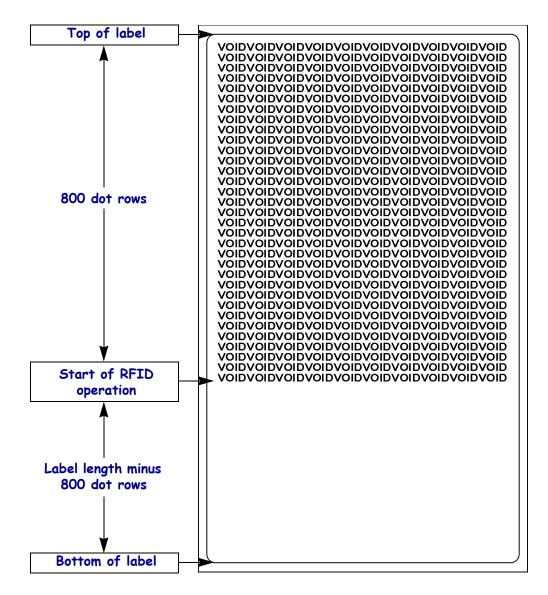
**Example 2** • This example sets the printer to move the media to 800 dots from the top of the media [or label length - 500 from the bottom (leading edge) of the media] and prints "void" 500 dots in vertical length (Y axis) in case of an error.
