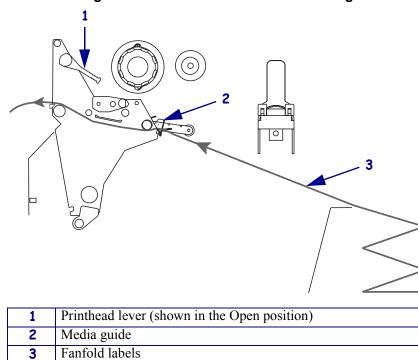
Figure 17 • Fanfold Media—Rear Loading
