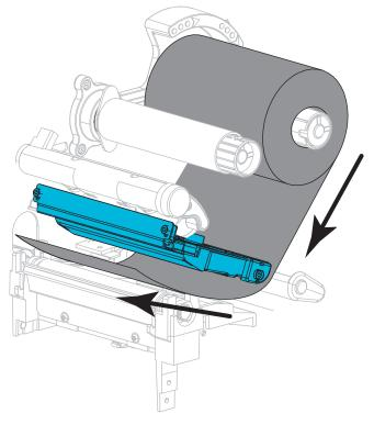
**4.** Bring the ribbon under the printhead assembly as shown.
