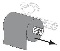
**3.** Discard the used ribbon. You may reuse the empty core from the ribbon supply spindle by moving it to the ribbon take-up spindle.
