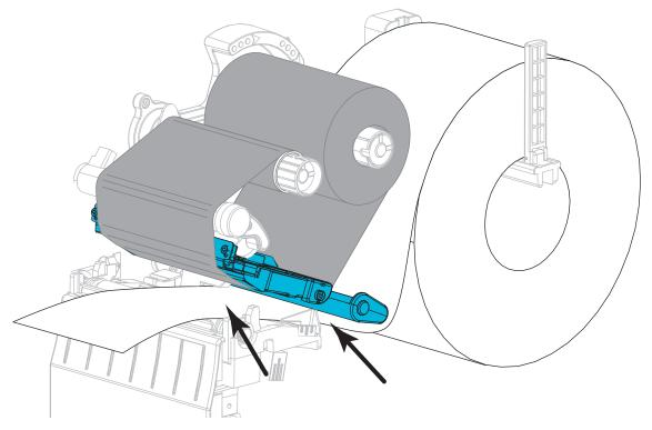
**13.** Make sure that the media passes through the slot in the transmissive media sensor (1) and under the inner media guide (2). The media should just touch the back of the transmissive media sensor slot.
