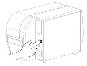
The printer boots up and performs a self-test. The results of the self-test are shown in Table 1 on page 8. If the media and ribbon are loaded correctly, the printer prints a printer configuration label (Figure 5) and then a network configuration label (Figure 6).
