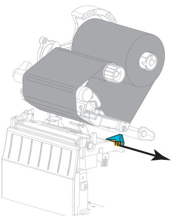
**12.** Slide the media under the media dancer assembly and the printhead assembly. Allow the end of the media to extend out of the front of the printer.
