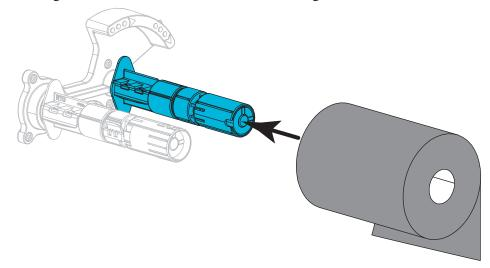
**3.** Your printer shipped with an empty ribbon core on the ribbon take-up spindle. If this core is no longer there, place an empty ribbon core on the ribbon take-up spindle. Push the core back as far as it will go.
