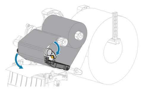
Rotate the printhead lever down to close the printhead.
