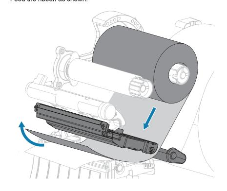
Wrap the ribbon around the core several times, and then rotate the spindle to tighten
